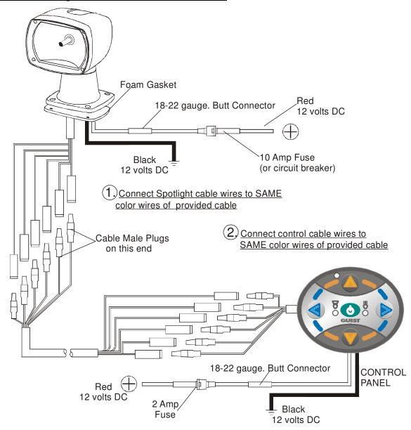
**Note:** When connecting to a 298-5 spotlight you will need to cut off the terminals, strip insulation back, and splice into existing control cable by matching the same color.
