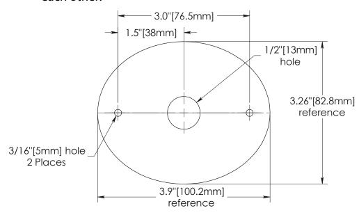
3. Feed all of the Control Panel wires through the center hole of the small gasket, then place the gasket underneath the control through the two threaded mounts.
