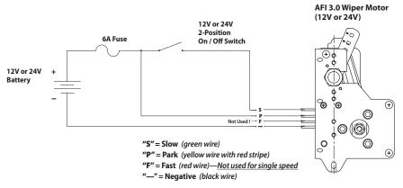
**Caution:** When wiring this two-speed motor as a single-speed you must use the slow speed as shown in the wiring diagram above and not the fast speed. Using the fast speed will ultimately cause the motor to over-heat and short out.
