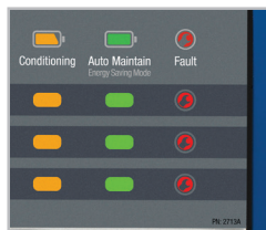
Battery fault detection LEDs
