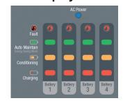
The ChargePro™ Series includes 1 Blue AC Power LED with 4 LEDs per battery bank with the following functions: Charging: Red Conditioning: Amber Auto Maintain: Green Fault: Red
