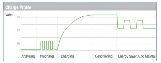
ChargePro's 5-Stage Performance Charging algorithm is fully automatic and designed to maximize battery performance and extend battery life.
